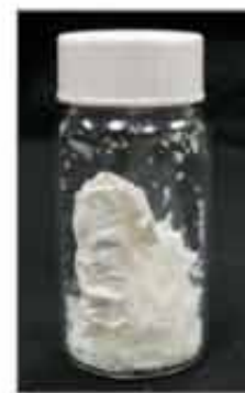
Figure 1. Bioplastic material produced using common bacteria.
