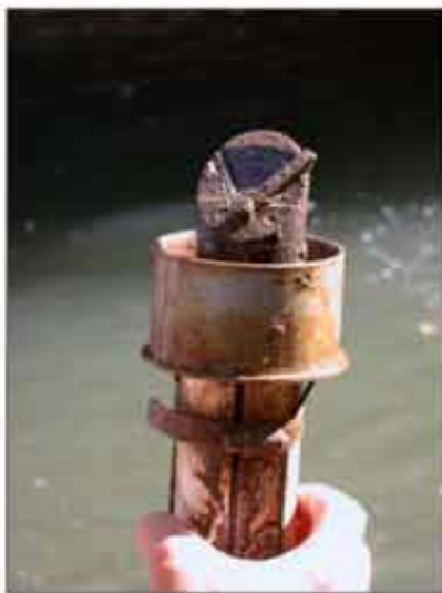
Sensor fouling is one challenge we are working to overcome in making reliable CDOM measurements.
