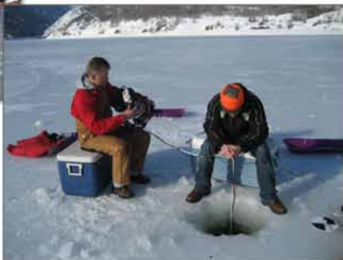
Figure 2. Light measurement through the ice on Pineview Reservoir
