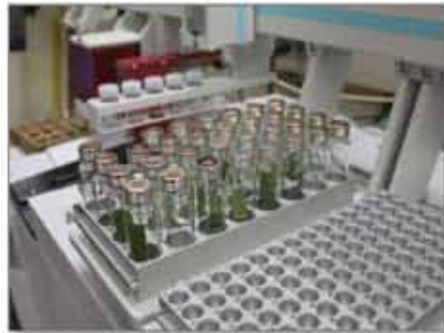
Headspace method for leaf-air partitioning
