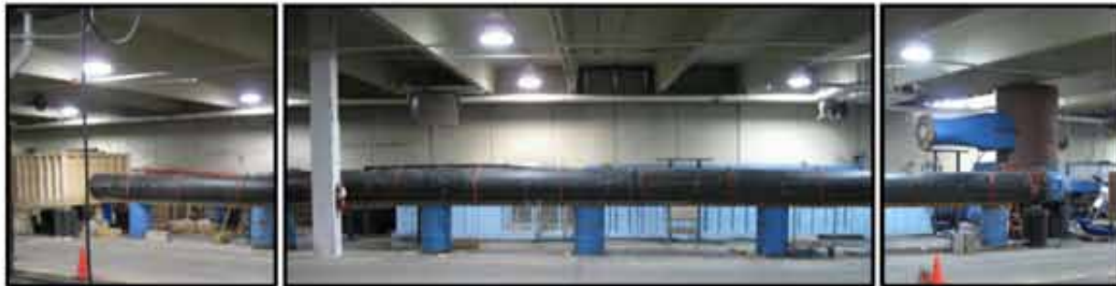
Baffled Culvert Test Set Up
