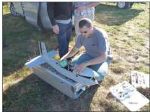
Modular design (easy for shipping as normal luggage in international travel as tested and verified in a real mission to New Zealand, 8/7 to 8/18/2012)
