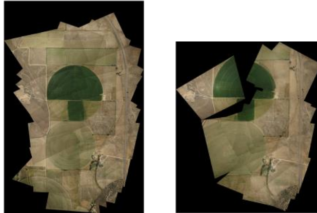
Figure 1. Mosaic maps generated from the aerial image set containing 158 images captured on June 17, 2013 by (left) using the high-resolution base map as a reference. (right) using the 2014 NAIP image as a reference. (Due to the difference of resolution in reference images, the sizes of the final mosaic maps are different.)
