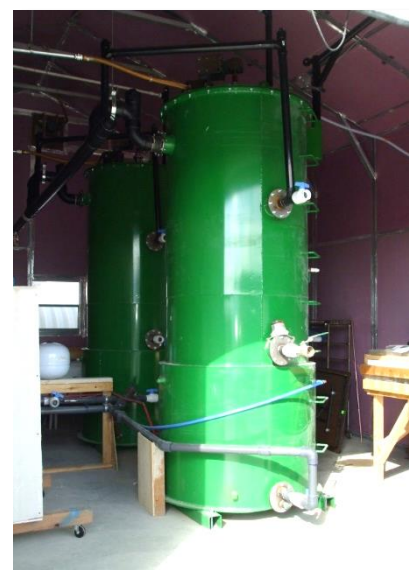
Figure 2. Upflow Anaerobic Sludge Blanket bioreactors for the production of biomethane from blending wastewater grown algae and carbon-rich wastes for production of heat and power
