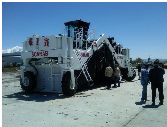
Figure 1. Sludge Compost Turner – Central Valley Wastewater Treatment Plant – Salt Lake City, Utah
