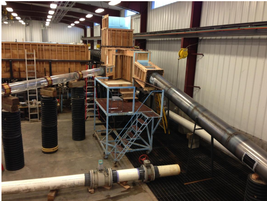
Physical model study of the Weber Basin Water Conservancy District's bifurcation structure
