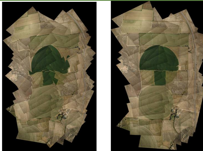
Figure 2. The mosaic maps generated from the aerial image set captured on June 17, 2013 by applying the direct georeferencing method on two kinds of data: (left) original GPS data. (right) updated GPS data.
