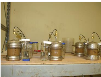
Figure 1. Set-up of small column study for testing sequential microbial processing of TCE under different conditions of biostimulation
