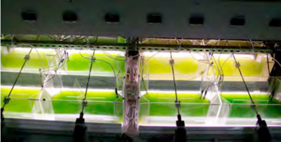
Figure 1. Laboratory raceway bioreactors designed and operated to improve algal growth and phosphorus uptake for treatment of the Logan Lagoon wastewater treatment system.
