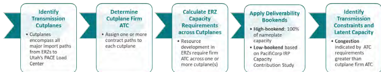
Figure 14: Methodology for Identifying Transmission Constraints
