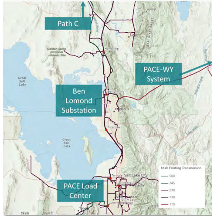
Figure 8: Power Grid in Northern Utah
