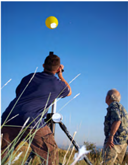
ValidWind™, a lidar-based balloon tracking system
