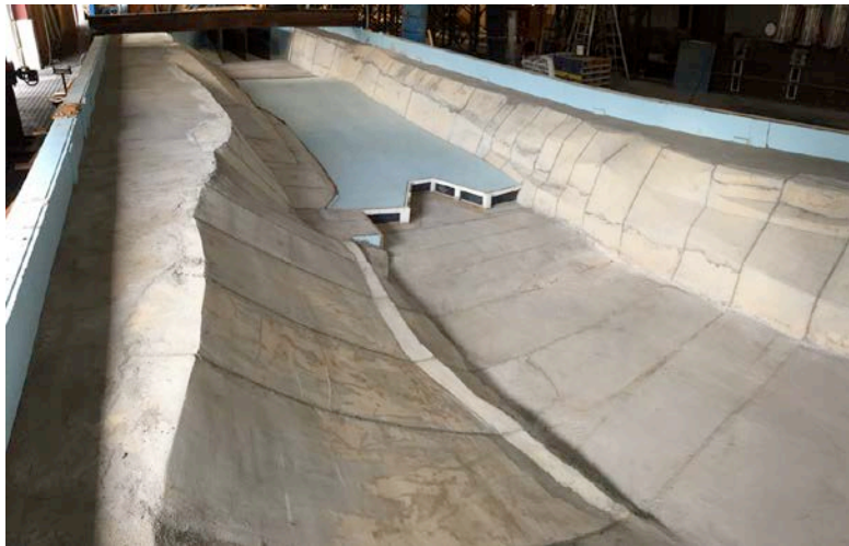
Physical model study of Virgin River Gorge Fish Barrier
