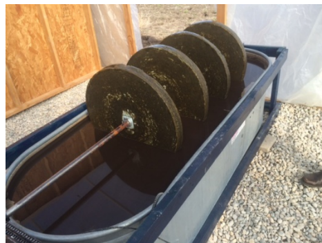
Figure 1. Rotating Algae Biofilm reactor at the Caine Dairy Farm using biofilm algae for wastewater treatment and bioenergy recovery through anaerobic digestion of algae biomass
