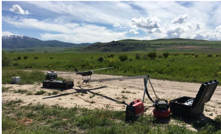
Figure 2. BluJay prototype ground system with launcher and control equipment, ready for takeoff
