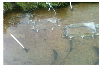
Figure 2. In Situ Benthic Chambers and Piezometers at the Silver Creek Field Site
