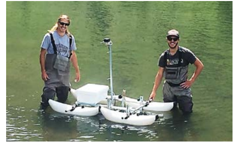
Figure 2. A mobile water quality monitoring platform enables us to examine spatial patterns in water quality that we cannot observe with grab sampling or fixed sensors
