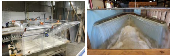
Figure 3. Large-scale piano key and labyrinth weirs
