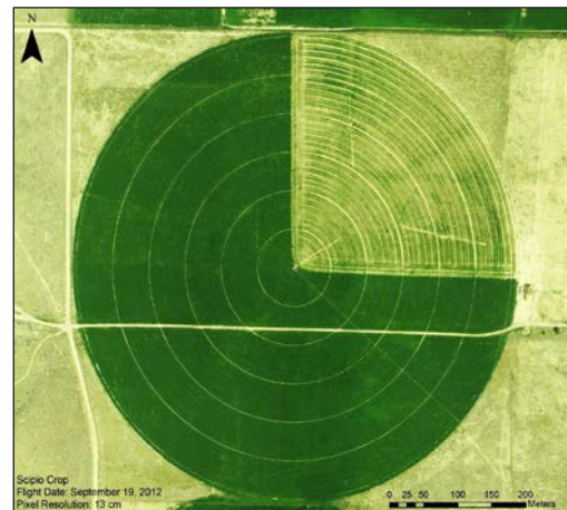
Aerial imagery of the center pivot system in Scipio obtained from UAV flights used to estimate soil moisture, evapotranspiration rates, and plant nitrogen content
