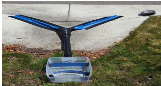
Figure 1. Curb flow meter installed at the 300 E site, Logan
