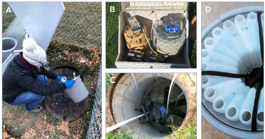
Figure 1: (A) Wastewater sampling at the main Logan campus, (B) autosampler used for wastewater monitoring, (C) typical manhole configuration for sampling of multiple housing units, and (D) bottles in autosampler units for sample collection over time.
