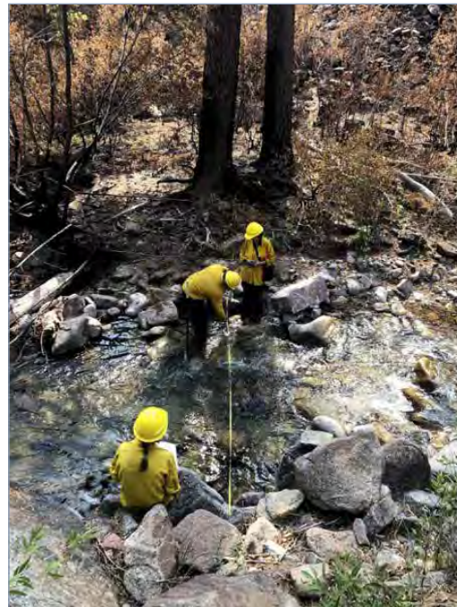
Figure 2: Lane's team is monitoring post-wildfire hydrologic response to track changes in streamflow and sediment dynamics in the Grizzly Creek Fire burn scar.
