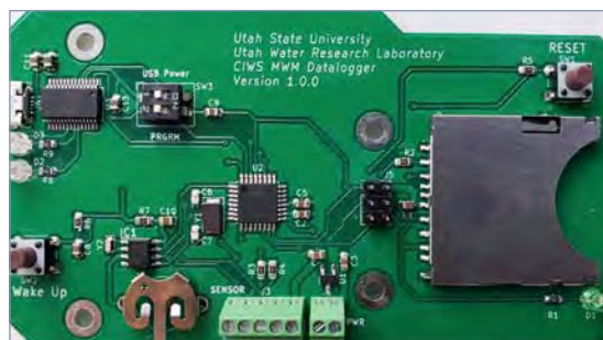
Figure 1: The custom smart water meter datalogger designed and developed by the project for collecting high-resolution water use data on existing residential water meters.
