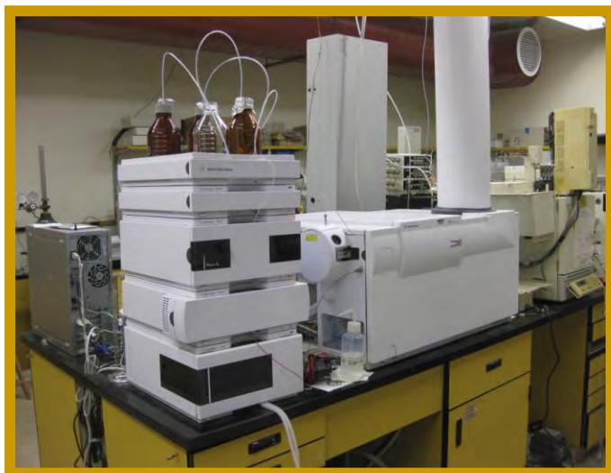
LC/ MS system for analysis of PPCPs
