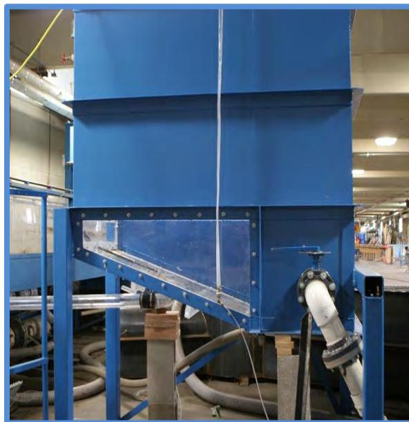
Lab-scale low-level outlet model.
