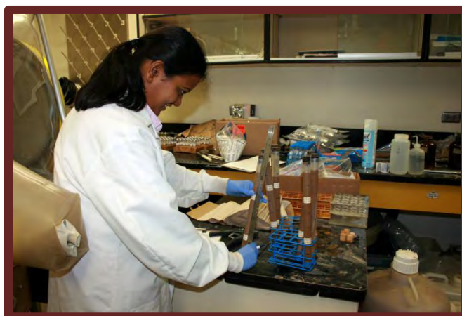
Figures 1 and 2. Processing the six-foot columns packed with aquifer solids for Hill AFB. Groundwater with TCE plus various carbon sources has been passed through the columns for over six years. The columns are now being sampled to investigate the biogeochemical processes that are favorable to TCE degradation.
