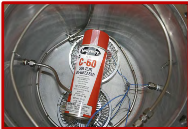
Emission chamber sampling of consumer de-greaser.
