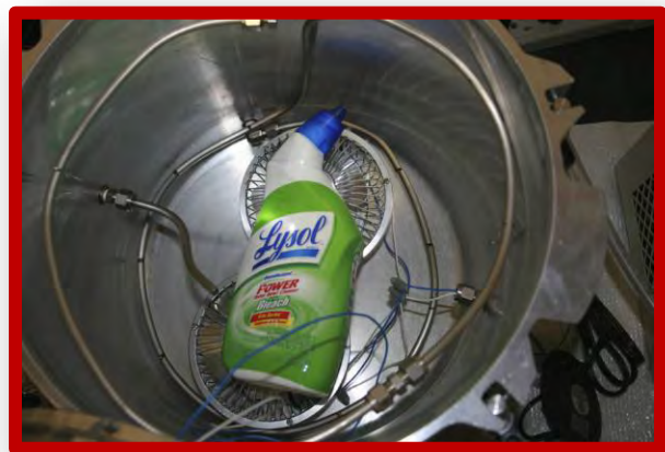
Emission chamber containing consumer product.
