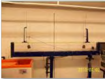
Figure 1. Two 20KHz acoustic transducers inside flume with flowing water at the Hydraulics Lab, Utah State University.
