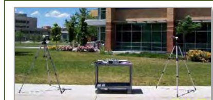
Figure 4. Demonstration of a battery operated station with transducers mounted on tripods and other instruments on cart.
