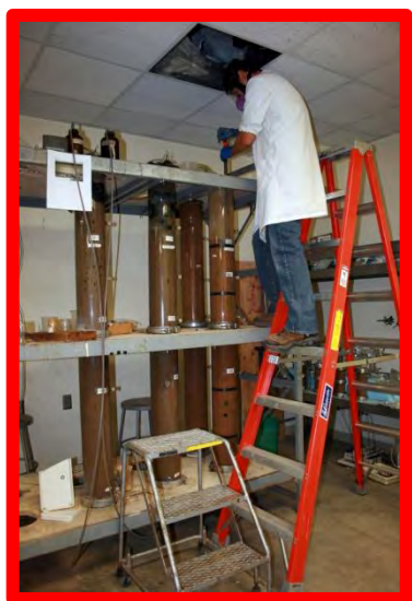
Figures 1 and 2. Processing the six-foot columns packed with aquifer solids for Hill AFB. Groundwater with TCE plus various carbon sources has been passed through the columns for over six years. The columns are now being sampled to investigate the biogeochemical processes that are favorable to TCE degradation.
