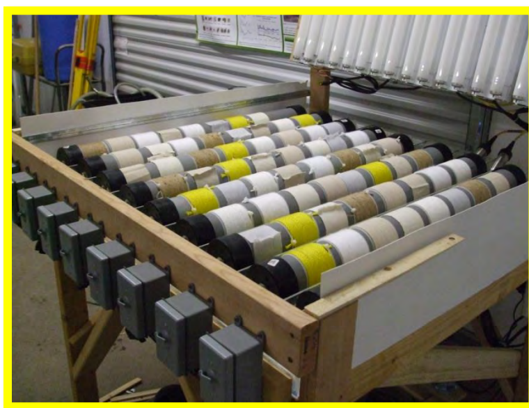
Figure 1. Rotating biofilm reactor materials tested to support algae growth included polyester, cotton, polypropylene, nylon, jute, and acrylic.
