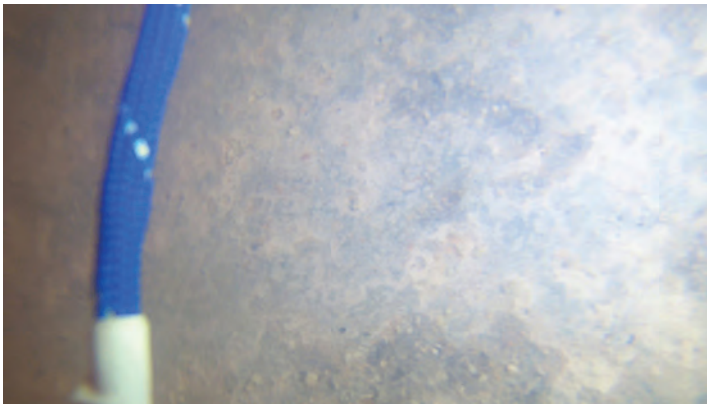
The salt crust on the floor of the north arm at a water depth of 10 feet in August 2019. The relatively smooth surface indicates that the crust is dissolving. The white segment of the cord is about 1 inch long.
