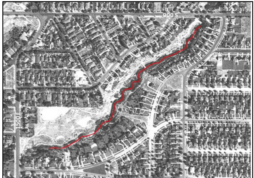
Figure 3.7. 1938 aerial photograph of Red Butte Creek from 900 South to 1500 East. Photograph is overlaid with 2006 channel alignment in red; gaps in line indicate underground culverts.
