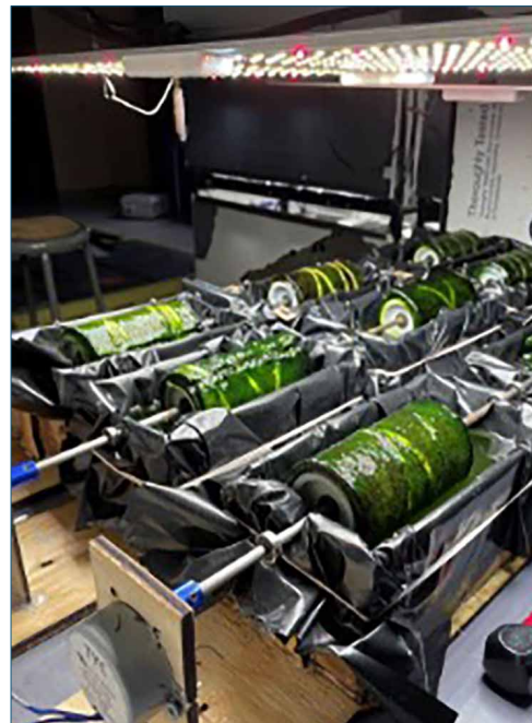
Figure 1: Testing unit for phosphorus removal from wastewater at the Central Valley Water Reclamation Facility in South Salt Lake City.
