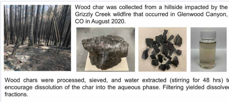
Figure 1: Sample processing to generate dissolved fractions of pyrogenic carbon samples collected from a real wildfire and lab-prepared chars.
