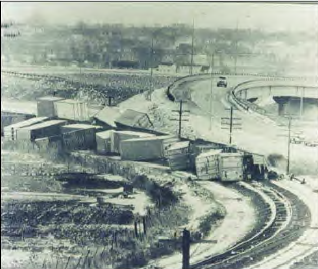
Wasatch Front, April 4-6, 1983 – 70 mph “East Winds” derailed this train in the Lagoon area. Peak gusts were recorded at 104 mph. Source: Utah’s Weather and Climate, Photo: Ogden Standard Examiner
