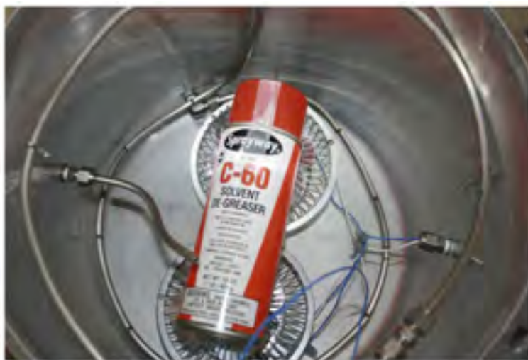
Emission chamber sampling of consumer product
