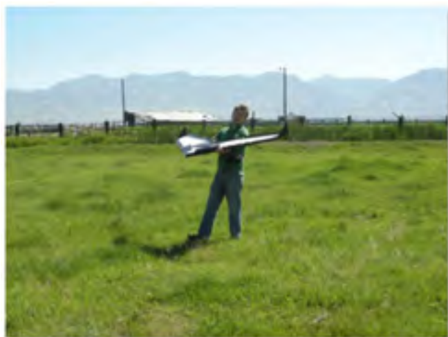
Figure 2. AggieAir™ remote sensing platform for algae monitoring in the Logan Lagoons operated by Austin Jensen of the Utah Water Research Laboratory
