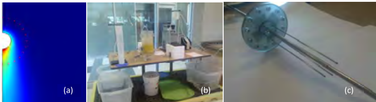
Figure 2. (a) Temperature profile of a probe of diameter 6.27mm. The red points are where the temperature-time curves are generated and are used to measure the thermal properties of the streambed. (b) Flow cell setup with penta-probe inserted (see picture "c"). The elevated cups allow the flow rate to be reliably adjusted. (c) Robust penta-probe. The center probe provides heating as well as a temperature response, and the four off set probes record temperature. The tip of the center probe is inserted 7" horizontally into the flow cell.
