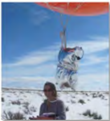
Portable ozone monitor attached to a tethered balloon
