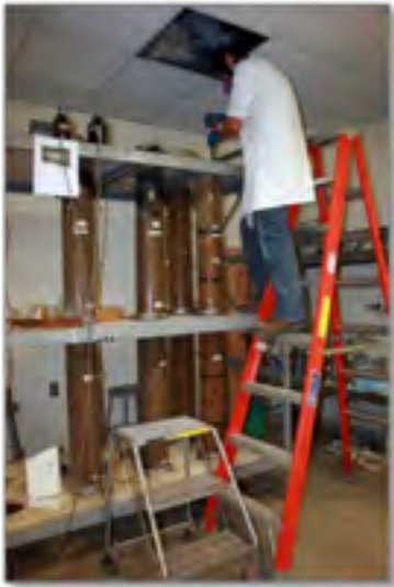
Figure 1. Processing the six-foot columns packed with aquifer solids for Hill AFB.
