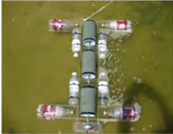
Figure 1. Zeolite-based rotating biofilm bioreactor in the Logan Wastewater Treatment Lagoon System
