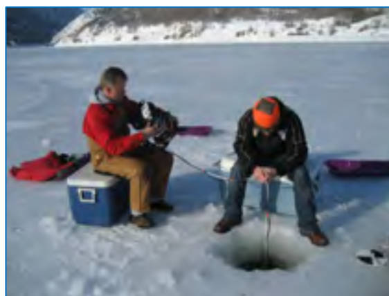
Figure 2. Light measurement through the ice on Pineview Reservoir
