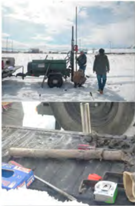
Figure 1. Collection of core material from the study site for evaluation of arsenic concentration through the profile and determining mineralogy of arsenic and biochemical processes of arsenic release to groundwater
