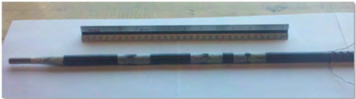
Figure 1. Large-diameter carbon fiber probe. The probe has depths of 3, 9 and 20cm, and will be used to measure the change in streambed thermal properties as a function of depth. This probe is robust enough to be pounded into a cobble streambed.
