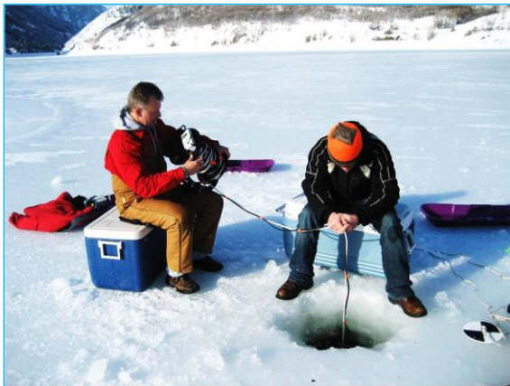
Figure 1. Light measurement through the ice on Pineview Reservoir
