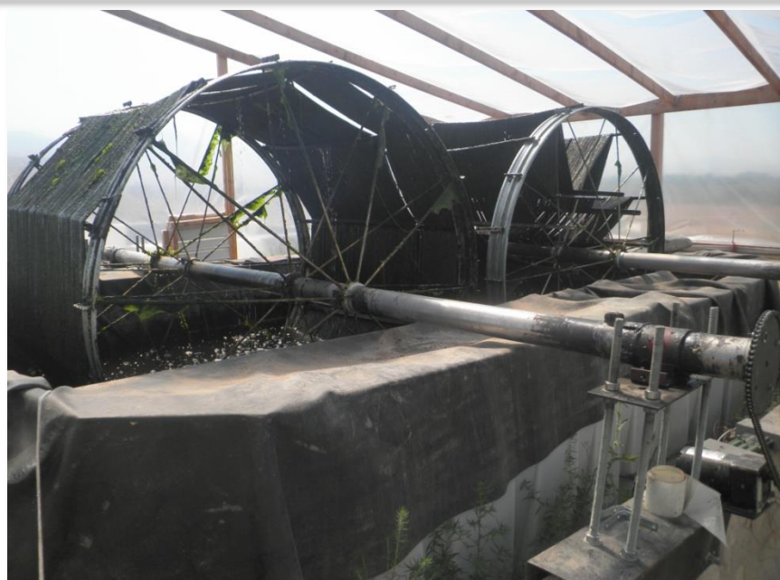
Figure 1. Rotating Algae Biofilm Reactor (RABR) with increased surface area for algae growth and increased phosphorus removal from Logan City Wastewater Treatment Lagoons wastewater.
