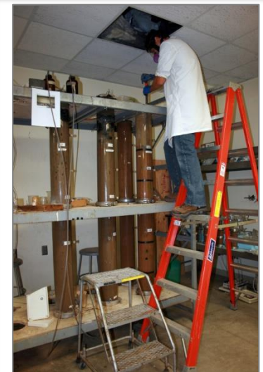
Figure 1. Processing the six-foot columns packed with aquifer solids for Hill AFB. Groundwater with TCE plus various carbon sources has been passed through the columns for over seven years. The columns are now being sampled to investigate the biogeochemical processes that are favorable to TCE degradation. But what happens to arsenic?
