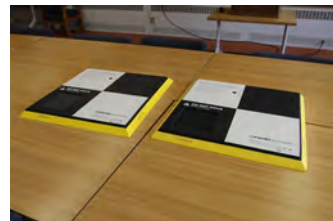
Propeller aeropoints aerial targets
