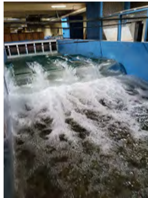
Scour morphology and foundation protection experiments at Utah Water Research Laboratory supporting general research and projects
