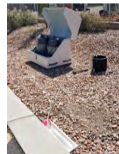
Figure 3: Sample collection at a stormwater BMP site, Salt Lake City Public Utilities building
