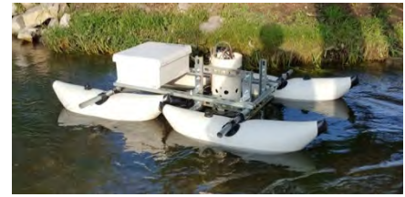
Figure 2. A mobile water quality monitoring platform enables us to examine spatial patterns in water quality that we cannot observe with grab sampling or fixed sensors
