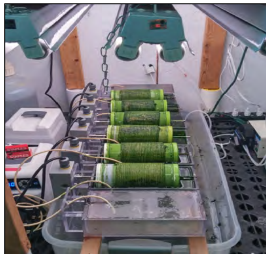
Figure 1. Rotating Algae Biofilm Reactor for laboratory testing of nutrient uptake from wastewater into microalgae biofilm
