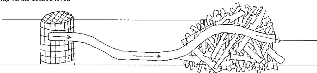
A pond leveler can be combined with a protective culvert fence in situations where the height of the roadbed is sufficient that a small beaver pond does not pose a threat. Ideally the pond should be left as large as is feasible without creating conflicts.
